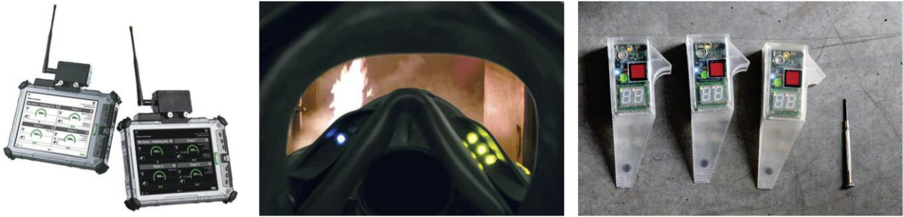
Figure 3. Illustrations for T5-T7: Transmission of air supply using “alphaCONTROL2” (left side 6 ), augmented reality breathing mask “alphaHUD” (middle 7 ), and “Landmarks” deployed as bread-crumbs for indoor positioning (right side, Ramirez et al. (2012))
