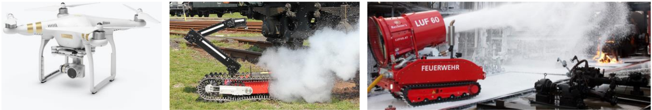
Figure 2. Examples for T3 and T4: UAV “Phantom 3” (left side 3 ), UGVs “taurob tracker” (middle 4 ) and “LUF 60” (right side 5 )
